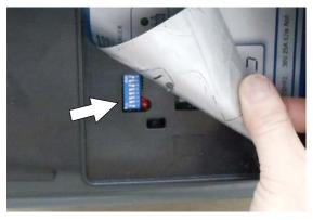
Set the switch positions according to battery type below.
